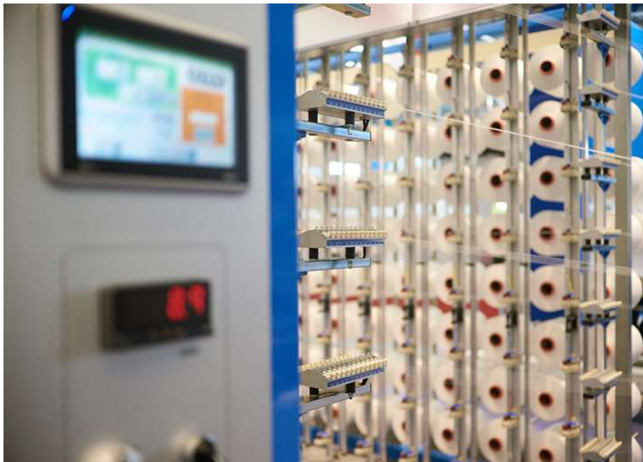
The Eltex EyETM monitoring yarn tension on a warping creel.
