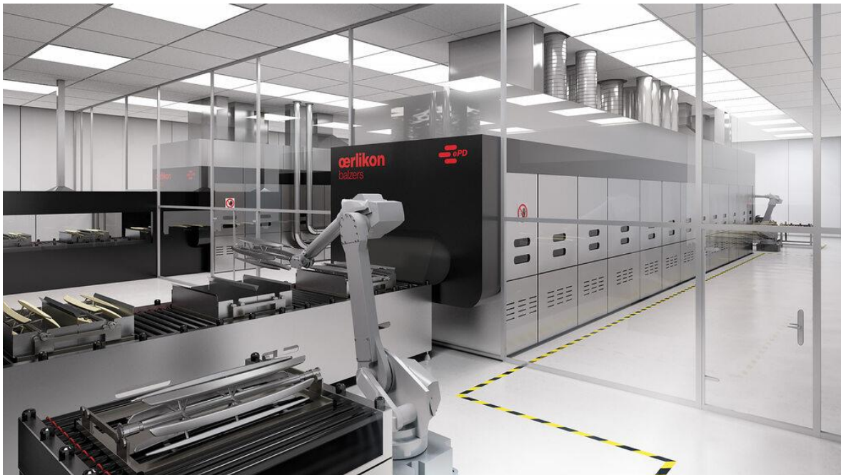
INUBIA I (ePD): Integrated equipment for the metallisation of plastics (ePD).
